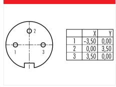
Contact arrangement (Plug-in side)
